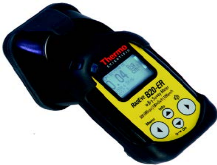
FIGURE 3.1: RADEYE B20-ER MULTI-PURPOSE SURVEY METERS
